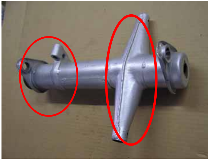
Fig. 5 Magnetic particle inspect for cracks and separation.
