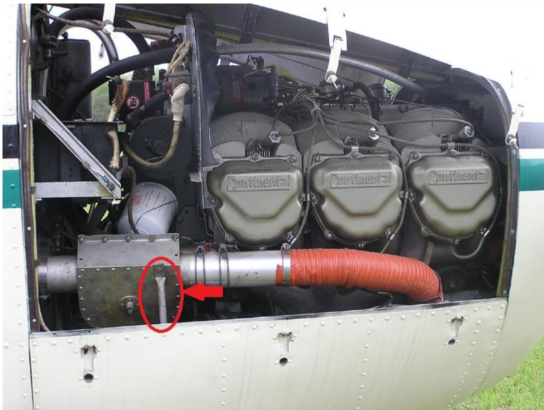
Figure 1. 147-30001/161-30001 Cowling Installation (No power plug installed). Red circle indicates support bracket (Part No.147-30001-149)
