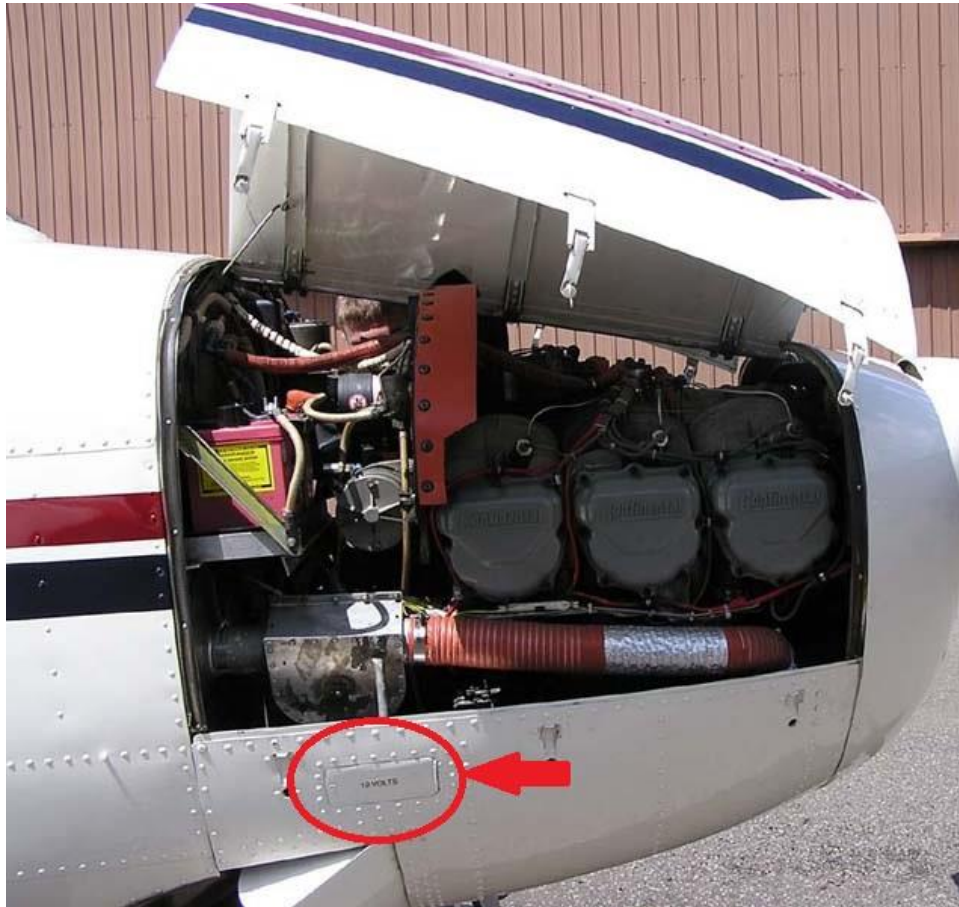
Figure 2. 147-30001/161-30001 Cowling Installation (with power plug installed). Red circle indicates power plug opening
