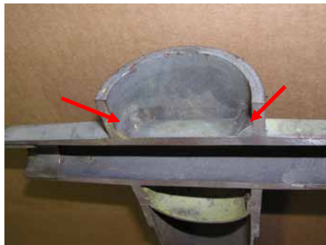
Fig. 7 Magnetic particle inspect for cracks and separation.
